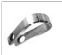
SOONV B-2 alloy Annealed + 1 hr at 1290°F (700°C) (Intergranular cracking, 3 hours)
